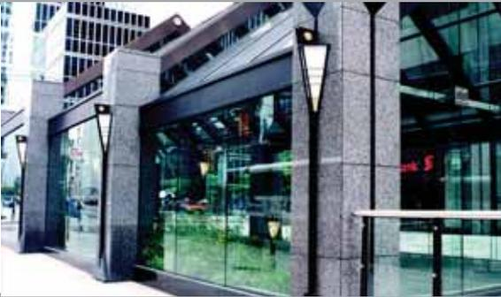
Custom, street-level outdoor wall mounted luminaires specifically designed and built to complement the architectural features of this commercial building with no visible fasteners or hardware.
